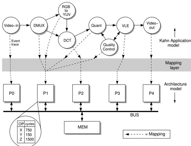
**Figure 1. Modeling an Motion-JPEG application on an MP-SoC architecture.**
