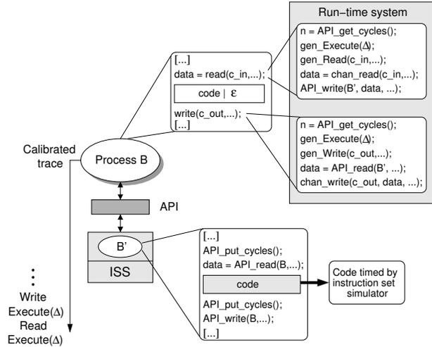
**Figure 3. Interaction between application model and instruction set simulator.**
