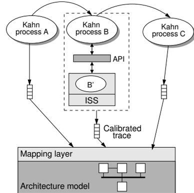
**Figure 2. Incorporating an instruction set simulator using trace calibration.**
